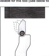
The cutter can be adjusted to suit the best position for the cut required. To start hollowing use the cutter in-line with the shaft and bore the centre of the box
