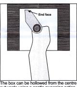
The box can be hollowed from the centre outwards using a gentle sweeping action. Adjust the cutter so that the end face cuts a flat bottom and neatly into the corner.
