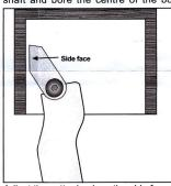
Adjust the cutter back so the side face is flat to create parallel sides to the box.
